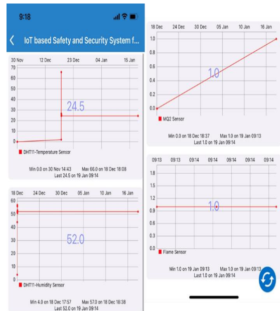
Figure 9: The Result of DHT11, MQ2 and Flame Sensors in the Thingview Program
